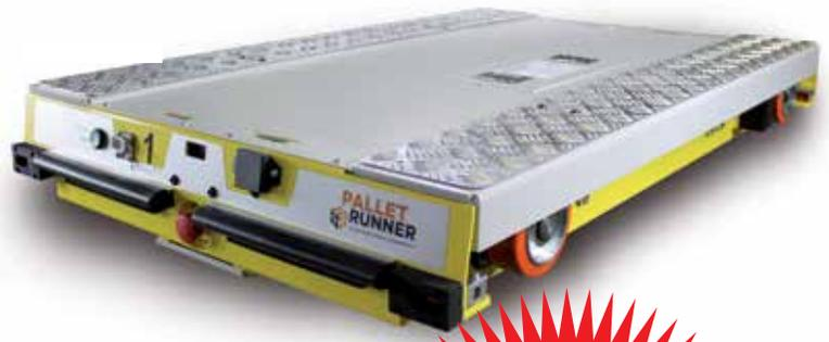
Pallets are unloaded and loaded into the system from the first or "Home" position at either end with a Pallet Shuttle Cart. The cart is designed to transport pallets being stored into the system, and retrieve the pallets as needed for shipment.
